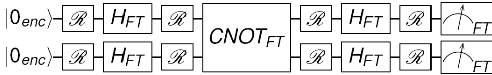
Figure 7.6: Example of a fault-tolerant circuit, with error recovery \mathcal{R} after every operation.
