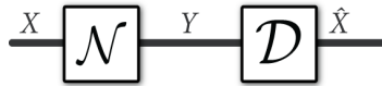
Figure 10.6: The classical communication scenario relevant in Fano’s inequality. Alice transmits a random variable X over a noisy channel \mathcal{N} , producing a random variable Y . Bob receives Y and processes it according to some decoding map \mathcal{D} to produce his best estimate \hat{X} of Y .
