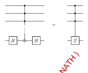
after conjugating the last bit by  $\boldsymbol{H}, \theta^{(n)}$  becomes controlled  $^{(n-1)}$ - $\boldsymbol{\sigma}_z$ , which flips the phase of  $|11...|1\rangle$  and acts to wally on all other computational basis states. Conjugating by  $NOT^{(n)}$ , we obtain  $\boldsymbol{U}_s$ , aside from an irrelevant overall minus sign.
